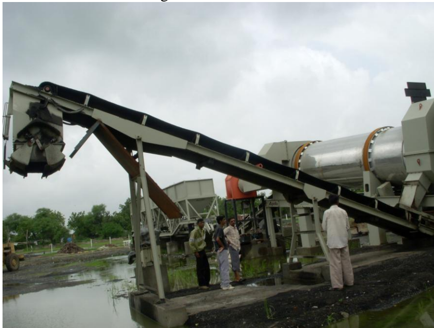
Fig. Load Out Conveyor
